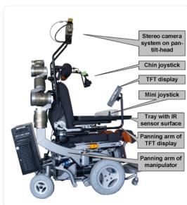
Figure 5-10: "FRIEND", care providing robot
